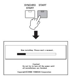
The version update is complete when the completion message below appears. Turn off the DDK-7 and disconnect the USB flash memory device.
