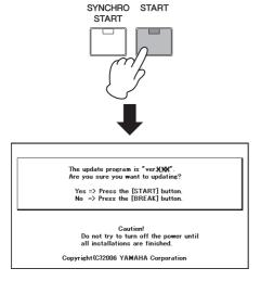
Confirm the version number to be installed, then press the [START] button to start installing the version update.
