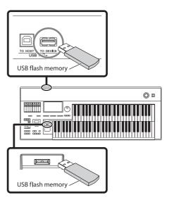
3. With the USB flash memory device containing the version update inserted/ connected, simultaneously hold down the [START] button in the Rhythm section on the panel and turn on the power switch.
