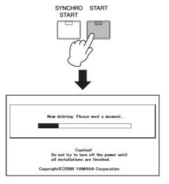
Make sure that you do not disconnect the USB flash memory device, or turn off the power during the Delete operation. Doing so may result in damage to the USB device.
