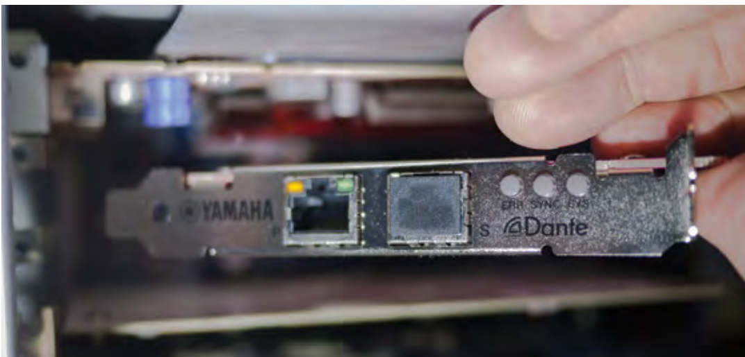
Figure 2.2 AIC-128 Dante Accelerator PCIe card being inserted
