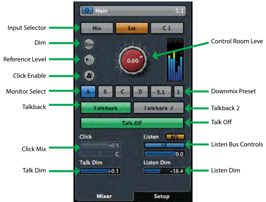
Figure 4.38 Control Room Main section
