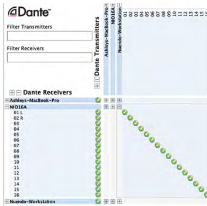
Figure 4.13 Routing 16 workstation outputs to the NI/O 16A
