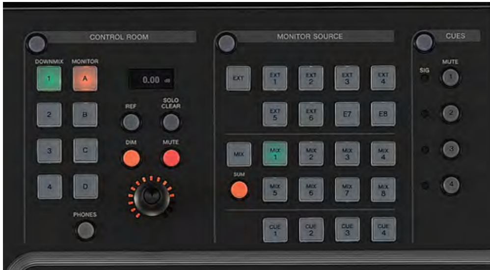
Figure 4.43 Master Unit Control Room sections
