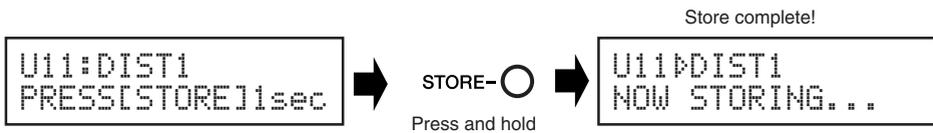
*\* To cancel the store operation, press and quickly release the [STORE] button (within 1 second) and the MAGICSTOMP returns to its original condition (the changed patch name returns to its original name).*
