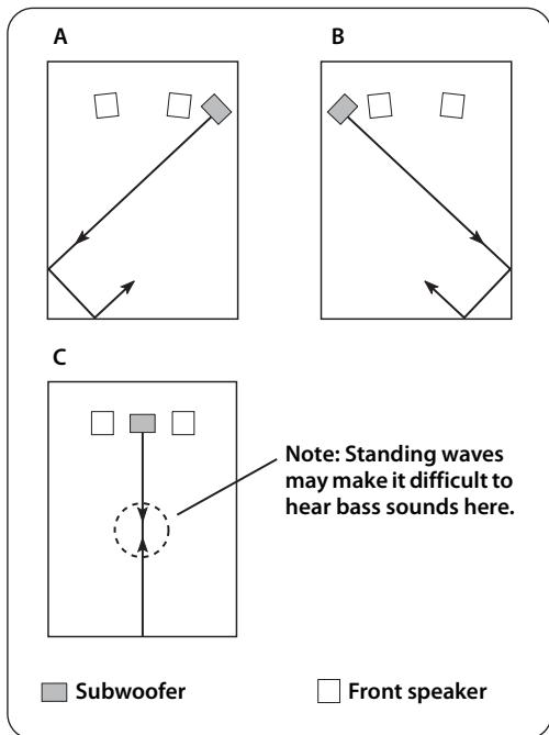
The placement shown in C is also possible, however, if the subwoofer is placed directly facing a wall and your listening position is in the center of the room, you may not be able to obtain enough bass sound from the subwoofer. This is because "standing waves" are forming between the two parallel walls and cancelling out the bass sounds. In this case, position the subwoofer at an angle to the wall. It may be necessary to break up parallel wall surfaces by placing bookshelves, etc., along them.
