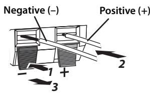
Note: Make sure the terminal is gripping the bare wire, not the insulation.
