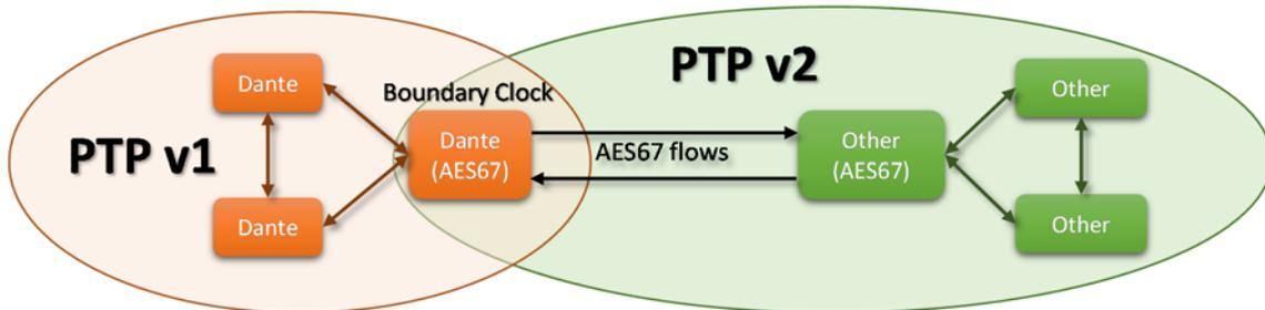
Dante and PTP v2 use different methods for electing the Master device. So when using the two in combination, care needs to be taken. Devices that support PTP v2 have many different priority levels available for becoming the Master device. Dante takes care of this automatically, while other PTP v2 devices may be configured manually. Select the most appropriate strategy for clock distribution, and follow these basic guidelines below.
