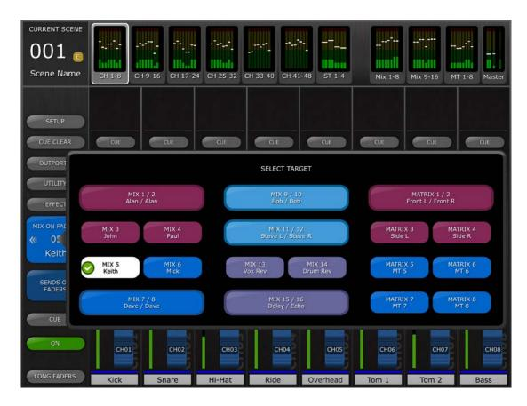
Select the Target from Mix 1-16 and Matrix 1-8. The currently selected Mix will appear as a white button with a check mark. Stereo pairs appear as single large buttons.
