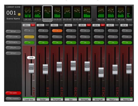
Faders can be moved to change the HA Gain for each channel. The gain value of each head amp will be displayed above the fader while any fader cap is being touched. Up to 8 faders can be adjusted simultaneously.
