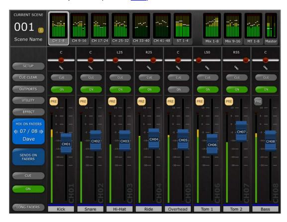
The large [MIX ON FADERS] button displays the currently selected Mix or Matrix Bus number and its name. The color of this button matches those used in the M7CL console.
